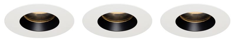
98mm (3.86") overall trimless diameter. Up to 45° loackable tilt and 350° lockable rotation. Supplied with standard trim kit. Family of matching products also available. Required depth height + 25mm^
