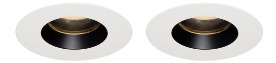
98mm (3.86") overall trimless diameter. Up to 45° loackable tilt and 350° lockable rotation. Supplied with standard trim kit. Family of matching products also available. Required depth height + 25mm^
