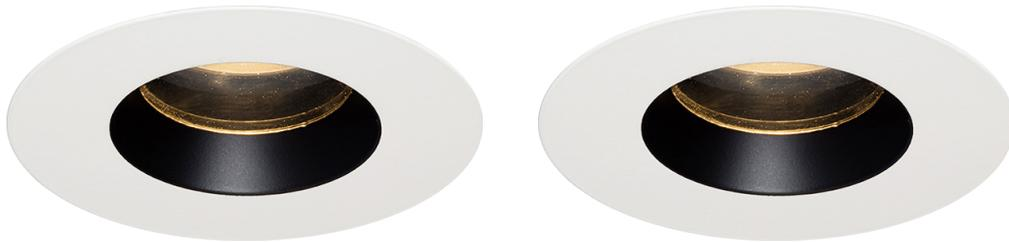
98mm (3.86") overall trimless diameter. Up to 45° lockable tilt and 350° lockable rotation. Supplied with standard trim kit. Family of matching products also available. Required depth height + 25mm<sup>^</sup>
