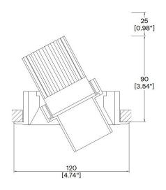
$\begin{array}{c} \text{A200/2-LS-LED-TR} \\ \text{Cut-out} \ 4.29 \text{"(109mm)} \ \varnothing \end{array}$
