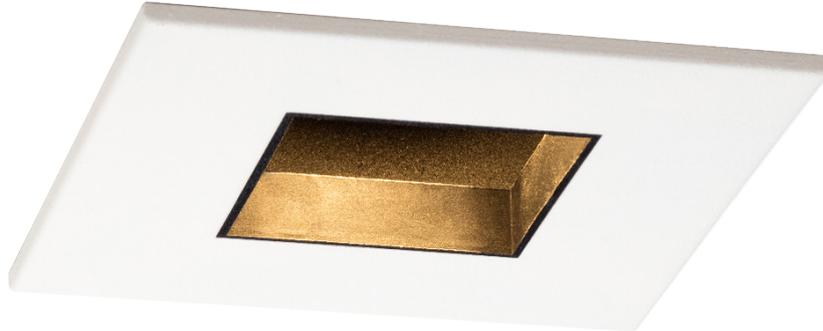
90 x 90mm (3.54 x 3.54") overall dimension. Shallow height downlight. Edge baffle to ensure aperture is glare free and for a professional look. Available with standard trim kit or plaster-in kit for flush appearance. Family of matching products also available. Required depth height + 25mm^
