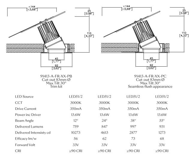
Apply these factors to 3000 K for lumen output of other CCTs:  $2200 \text{K} \times 0.65 / 2400 \text{K} \times 0.69 / 2700 \text{K} \times 0.98 / 4000 \text{K} \times 1.02$ .
