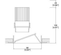
$\begin{array}{c} A090 + LED - TL - WW \\ 0^{\circ} - 30^{\circ} \ vertical \ adjustment \\ Cut-out \ 102mm \ (4.02") \ \varnothing \end{array}$
