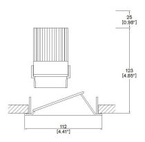
A090+LED-TR-WW 0° - 30° vertical adjustment Cut-out 102mm (4.02") Ø
