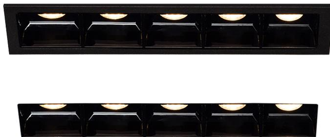
Line is a range of miniature ultra low glare recessed downlights with 1, 2, 5 or 10 cells. In fixed in a flanged or trimless installation kit. Available in 3 color temperatures and 3 beam angles. TRIAC/Phase, 0-10V/1-10V, DMX and DALI/digital dimming.
