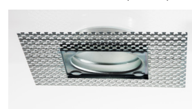
A31433-A-LED + 3000-PCZ 360° rotation. Up to 35° tilt. Cut-out 98mm (3.85”) Ø
