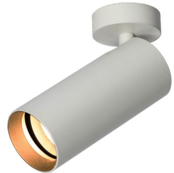
40mm (1.57") overall diameter. Miniature low voltage LED tubular spotlight. Available with monopoint mounting or magnetic track adaptor. Family of matching products also available.
