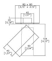
6100-LED-TMP Cut out 35mm Ø
