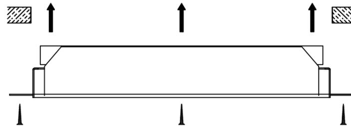
Fit the installation trim into the hole, square up trim as required and fix the frame to plasterboard with screws. *(Recommended - for additional strength bond trim into the hole).*
