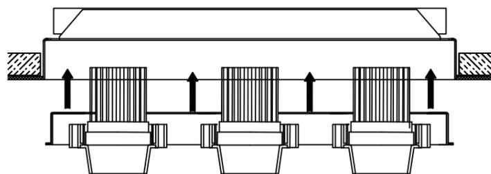
Install the gimbal cartridge into the installation kit.
