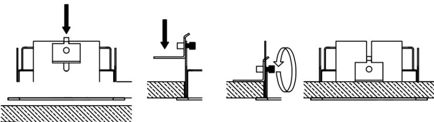
The fixing bracket(s) are installed in the slots at the short ends of the Gimbal housing as illustrated above. Finger tighten the knurled bolt, and securely tighten with an Allen (Hex) key after checking the Gimbal is sitting correctly in the cut-out and against the ceiling.
