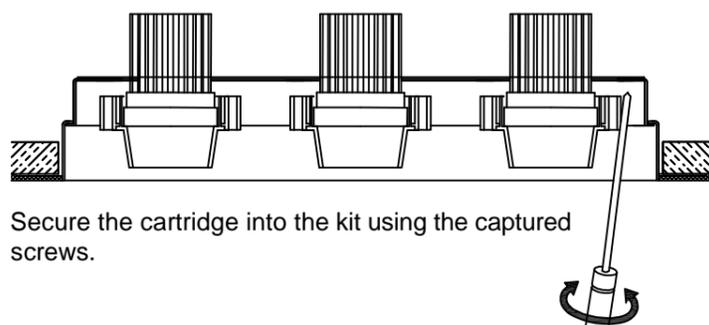
Secure the cartridge into the kit using the captured screws.
