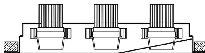
Install the Gimbal cover plate, the plate is held in by magnets.
