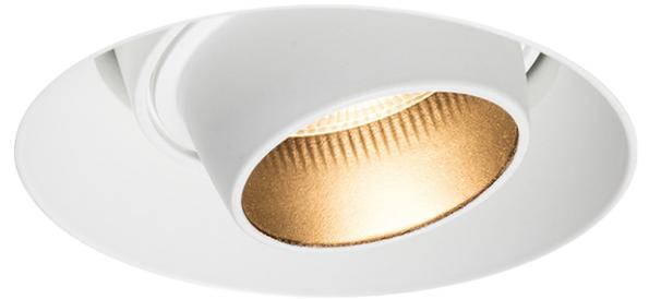
154mm (6.06") overall trim diameter. 127mm (5") overall trimless diameter. Available with standard trim kit or plaster-in kit for flush appearance. Family of matching products also available. Required depth height + 25mm<sup>^</sup>
