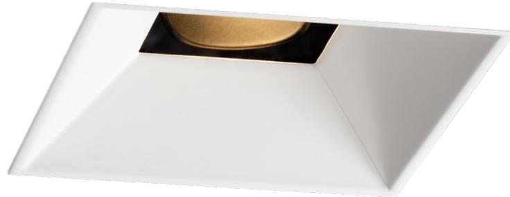
98 x 98mm (3.86" x 3.86") overall trim dimension. Manual adjustment tilt and rotation. 360° rotation. Up to 45° tilt. Available with standard trim kit or plaster-in kit for flush appearance. Family of matching products also available. Required depth height + 25mm<sup>^</sup>
