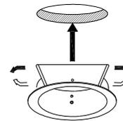
To install the ceiling trim into the ceiling, press spring blades toward the body and carefully insert into the ceiling cut-out. Push the luminaire up until trim is flat against the finished ceiling.
