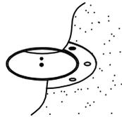
Skim plaster to the lip edge of the plaster ring. Make good and paint ceiling before installing luminaire body, cleaning any stray plaster from the trim.
