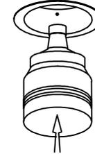
Install the luminaire housing into the ceiling ring, until the ball catches in the trim locates into the groove in the luminaires body. Fixture will sit flush with the finished ceiling.
