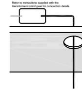
Connect transformer/control gear and insert through the ceiling ring.
