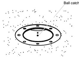
Fit the installation collar and fix to plasterboard with screws.
