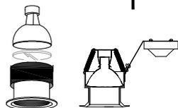
Install control gear/transformer where applicable through the ceiling cut-out. Wire equipment according to the installation instructions provided/printed on the equipment to the terminal block mounted on fixtures bracket. *(For GU10 versions please take mains supply directly to the plug/socket provided).*
