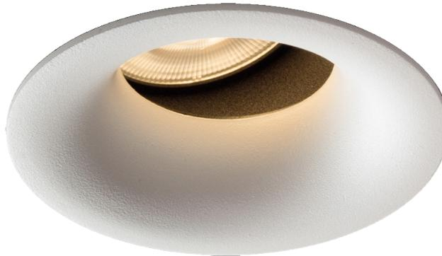
92mm (3.62") overall diameter. 360° rotation. Up to 30° tilt. Available with standard trim kit or plaster-in kit for flush appearance. Family of matching products also available. Required depth height + 25mm<sup>^</sup>
