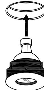
Install luminaire body into the ceiling ring until ball-catches locate in the trim's ball-race.
