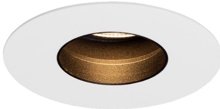
92mm (3.62") overall diameter. 360° rotation. Up to 30° tilt. Edge baffle to ensure aperture is glare free and for a professional look. Available with standard trim kit or plaster-in kit for flush appearance. Family of matching products also available. Required depth height + 25mm^
