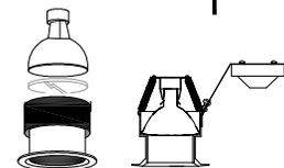
Install control gear/transformer where applicable through the ceiling cut-out.
