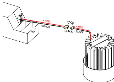
Install LED Drivers through the ceiling cut-out\*.
