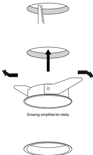
Fit the installation kit into the ceiling, press spring blades toward the body and carefully insert into the ceiling cut-out. Push the installation kit up until trim is flat against the finished ceiling. (Tip, for additional strength bond the ring into the ceiling).
