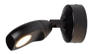
32mm (1.97") overall diameter. IP65 constant voltage exterior grade surface mounted fully adjustable ultra wide flood light. 90° Pivot and 359° rotation.
