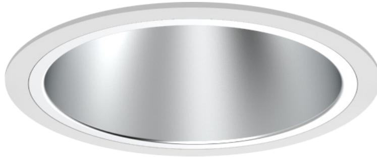
195mm (7.68") overall diameter dark light fixed downlight fixture. Supplied as standard with semi-specular silver reflector and white die-cast trim. Pattress provided for soft tile or metal ceiling installation. Suitable for installation into plasterboard ceiling upto 25mm thick. Required depth = height + 25mm<sup>^</sup>
