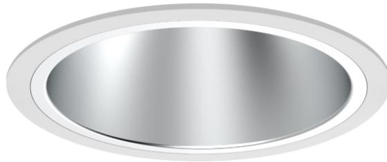
140mm (5.51") overall diameter dark light accent downlight fixture. Up to 35° tilt. Supplied as standard with semi-specular silver reflector and white die-cast trim. Pattress provided for soft tile or metal ceiling installation. Suitable for installation into plasterboard ceiling upto 25mm thick. Required depth = height + 25mm<sup>^</sup>
