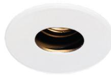
40mm (1.57") overall diameter. Fully recessed Micro40 downlight for interior installation. Available with standard trim kit or plaster-in kit for flush appearance. 20° with standard ceiling thickness with no chamfer (Diagram 1), 35° tilt max with chamfered ceiling (Diagram 2), When using trimless kit max tilt 10° (Diagram 3). Family of matching products also available. Required depth height + 10mm^
