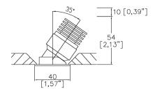
Diagram 2 M43-SA-TR Cut-out 36mm Ø
