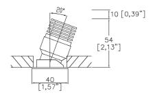
Diagram 1 M43-SA-TR Cut-out 36mm Ø
