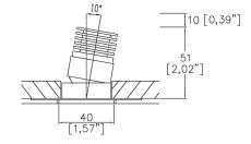
Diagram 3 M43-SA-TL Cut-out 37mm Ø
