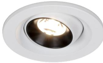
40mm (1.57") overall diameter. Max tilt 30°. Fully recessed Micro40 downlight for interior installation. Family of matching products also available. Required depth 25mm<sup>^</sup>
